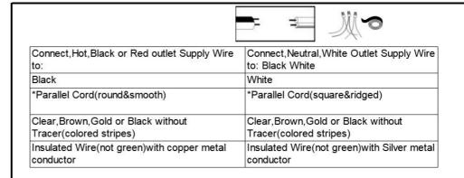
STEP2: To connectfixture wires: Connectthe live wire (L) from fitting to the live wire from main powersupply. Connectthe neutral wire (N) from fitting to the neutral wire frommain powersupply.make the wire connector(HW3) connect the ground wire. Please pay close attention to avoiding the wires exposingoutside when wiring connections.
