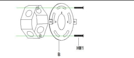
**STEP1:**Firstly install the Mounting Plate (B) with the (HW1) screw into the junction box.
