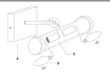
STEP4:Securely install the Light bulb (D) to the socket (C).
