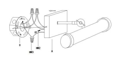
STEP3:Fasten the Mounting Plate (B) through the Lamp Body (A) with a screw (HW2)
