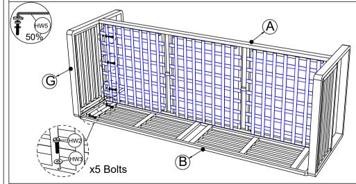
**STEP 3**: Connect Part from Step 2 & Right Armrest (G), tighten Bolt (HW2), Flat Washer (HW3) with Allen Key (HW5).
