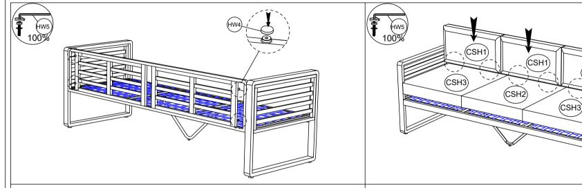
**STEP 5**: Firmly, tighten the Bolts. Put the Bench upright.
