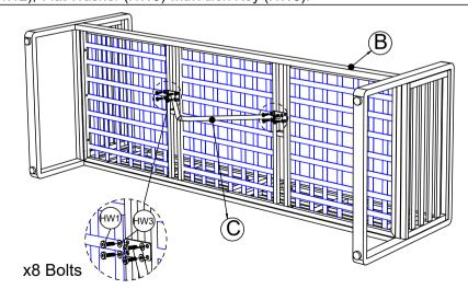
**STEP 4**: Connect part from step 3 & Support Leg (C), tighten Bolt (HW1), Flat Washer (HW3) with Allen Key (HW5).
