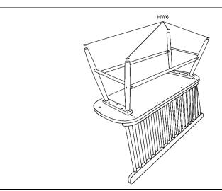
Step 4: PUT FELT PAD (HW6) TO THE BOTTOM LEG.
