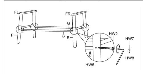
**Step 1:** INSERT JCBC (HW2) AND BARREL NUT (HW5) IN HOLE ON STRETCHER (D) TO ATTACH RIGHT LEG FRAME (D) AND LEFT LEG FRAME (E) THEN PUT WOOD BUTTON (HW7).
