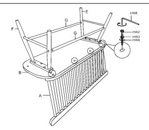
**Step 3:** USE JCBC (HW2) THEN PUT THE WASHER (HW2, HW3) TO ATTACH BACKREST (A).
