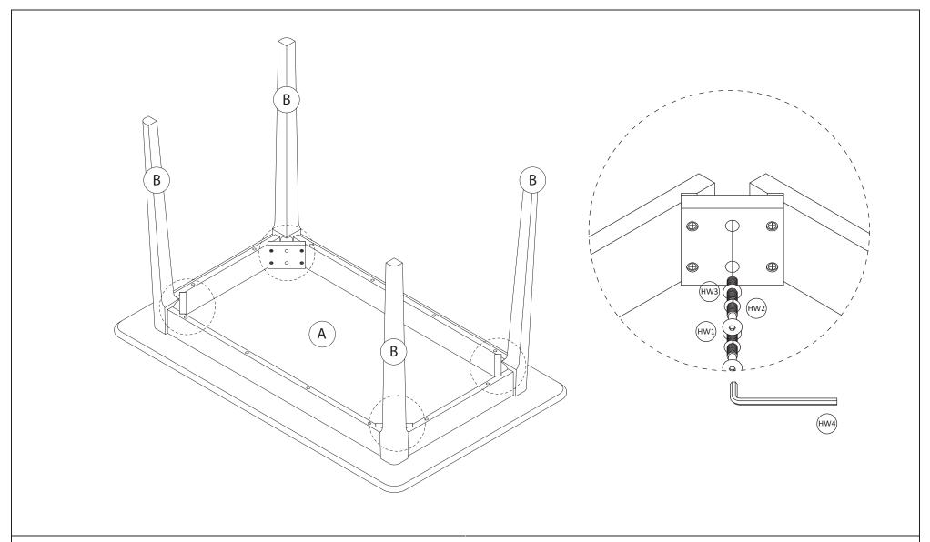
Step 1: Place the Table Leg (B) in position and screws in the bolts (HW1). Put washer (HW2,HW3) on the bolts (HW1) in the order shown in the picture.
