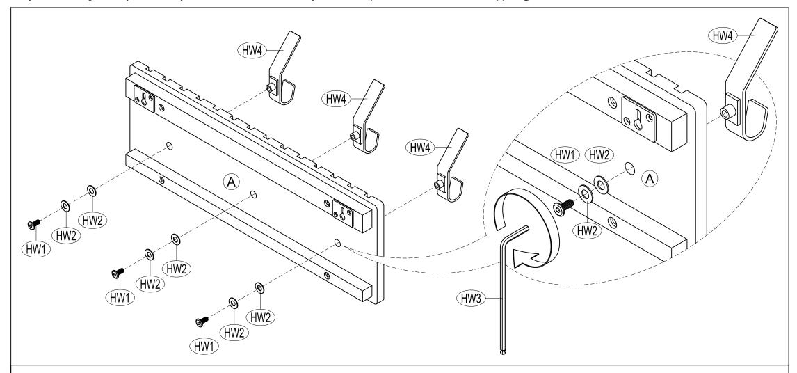
STEP 1 ATTACH HANGER (HW4) TO PANEL HANGER (A) USING BOLTS (HW1) AND FLAT WASHERS (HW2). TIGHTEN BOLTS (HW1) USING ALLEN KEY (HW3).
