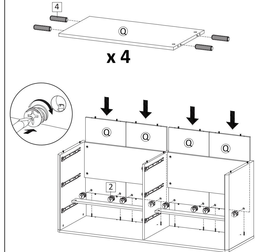
**STEP23:** Insert Dowel Ø8x30mm into Back Board (Q). Attach Back Boards (Q) into Top Board(A). Insert Camlock (HW2) then tighten using screwdriver as picture.
