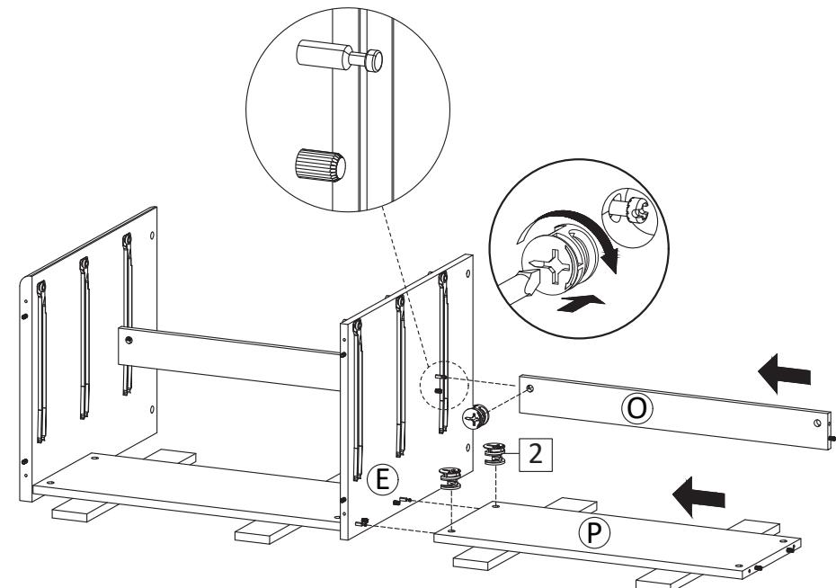
**STEP19:** Attach Support Board 1 (O) Support Board 2 (P) to the Center Board (E) from step 15. Secure with Camlock Big (HW2) and tighten it using screwdriver as figure.
