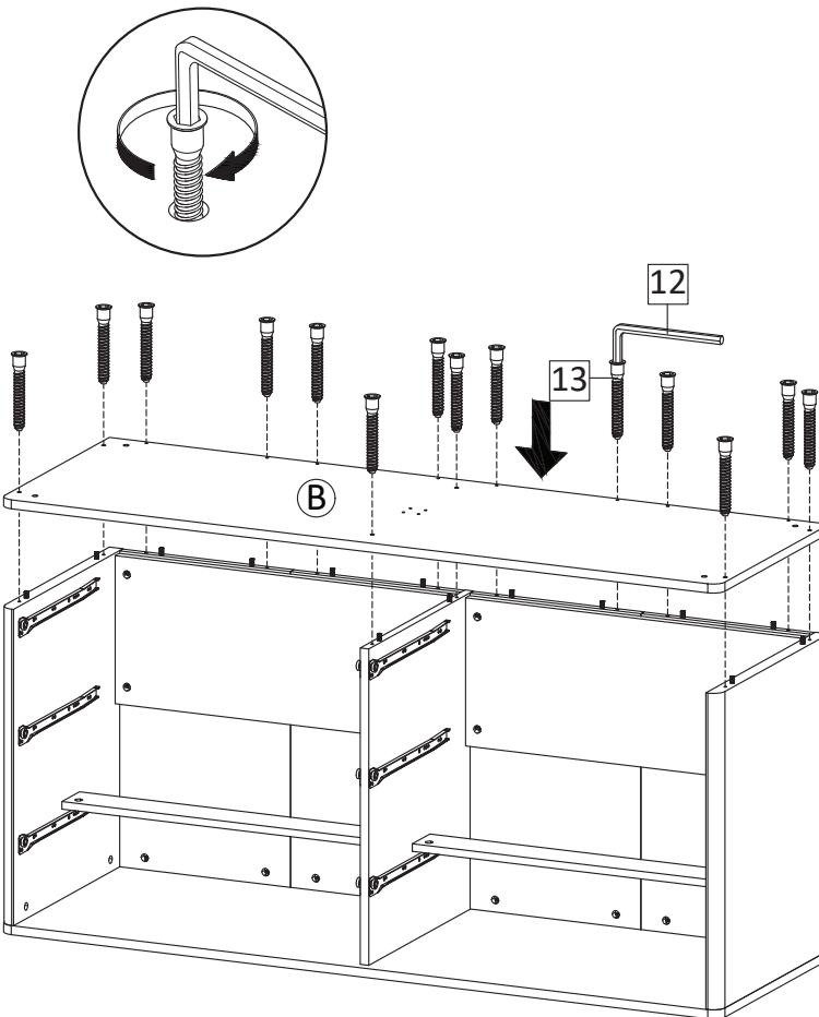
**STEP24:** Insert Bottom Board (B), secure with Screw M7x50mm (HW13), tighten screws using Allen Key (HW12).
