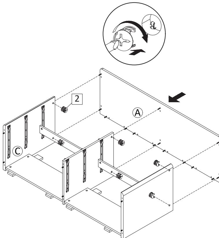
**STEP22:** Insert Top Board (A) and secure with Camlock Big (HW2) then tighten using screwdriver.
