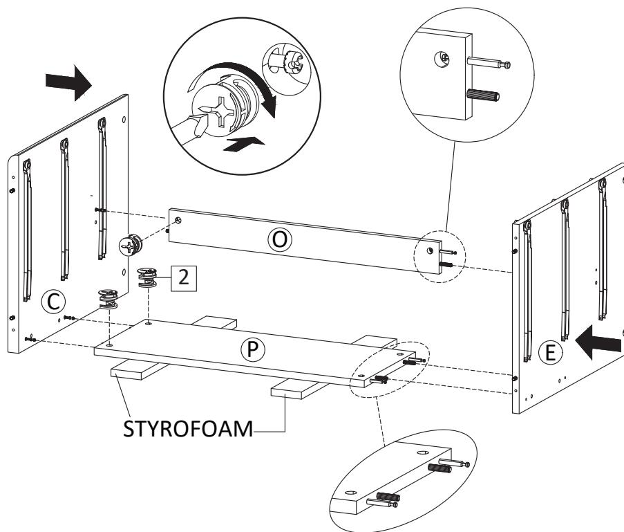
**STEP18:** Attach Side Board Left (C),Center Board (E) ,Support Board 1 (O) Support Board 2 (P). Secure with Camlock Big (HW2) and tighten it using screwdriver as figure.
