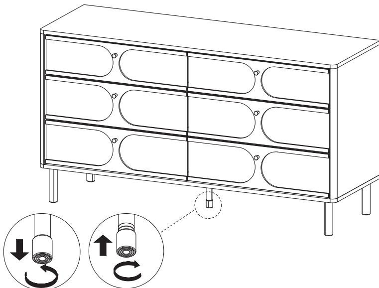
**STEP28:** Place your furniture on level floor. The legs come with adjustable leveller,adjust it as needed until your furniture sit steady on the floor. Assembly is complete.
