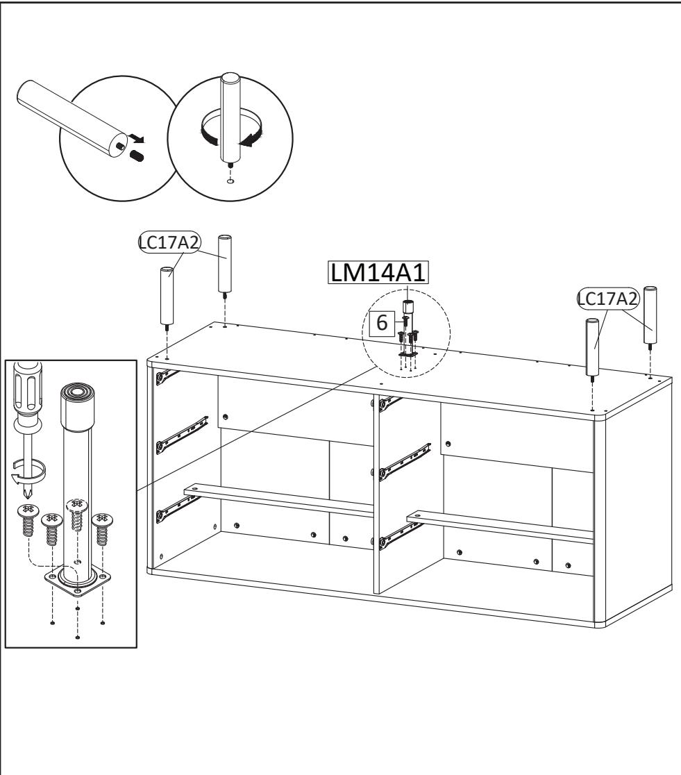
**STEP25:** Insert Leg (LC17A2) into position as shown in picture, tighten by rotating the leg clockwise. Install Metal Leg (LM14A1) secure with Screw M4.5x12.5mm (HW6) and tighten it using screwdriver as figure.
