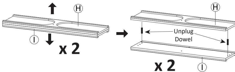
Remove the installed Dowel and do not use it again.
