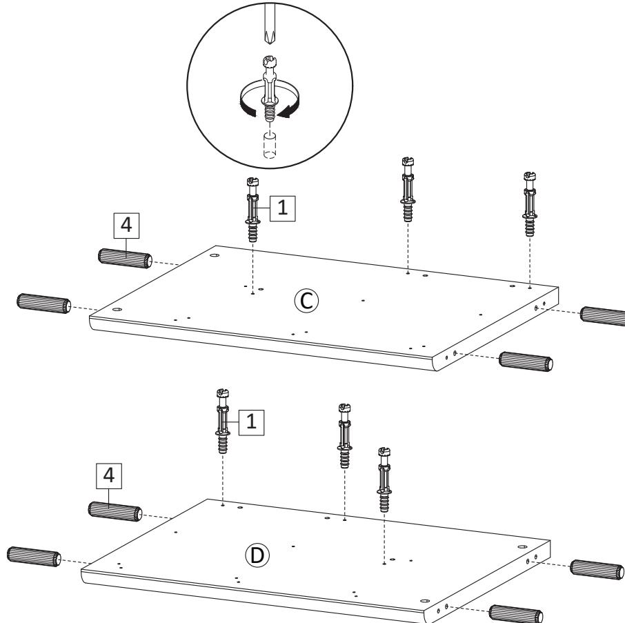
**STEP13:** Insert Dowel Ø8x30mm (HW4) into Side Board Left (C), Side BoardRight (D). Insert Cambolt Long (HW1) into Side Board Left (C), Side Board Right (D) into position as the above image.
