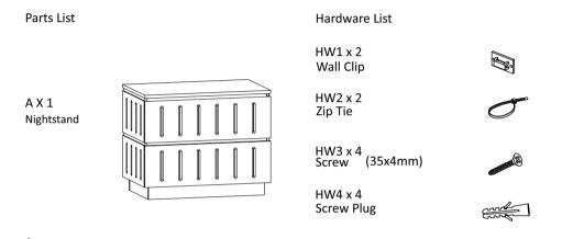
Insert the Screw Plugs (HW4) into the wall. Align the screw holes on the Wall Clip (HW1) to the Screw Plugs (HW4) in the wall. Use a screwdriver (not included) to screw in the screws (HW3).
