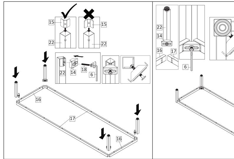
**STEP17**: Insert Support Corner Brace (HW15) and place it inside Leg (HW22) tube. Insert Screw (HW18) into the hole of Corner Brace (HW14). Screw in slightly just enough to grip Leg (HW22) with Support Corner Brace (HW15) inside Do not tighten. Arrange Support Metal Leg 1 (HW16) & Support Metal Leg 2 (HW17) on the floor as per image.
