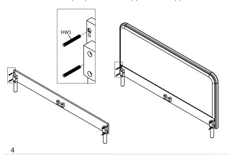
Attach the side rails (E) to the headboard (A) and footboard (B) by placing the metal threads through the holes on the side rails (E). Screw the semicircle washers (HW2) onto the metal threads. Then use the spanner (HW4) to screw on the nuts (HW3).
