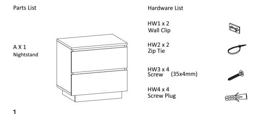
Insert the Screw Plugs (HW4) into the wall. Align the screw holes on the Wall Clip (HW1) to the Screw Plugs (HW4) in the wall. Use a screwdriver (not included) to screw in the
