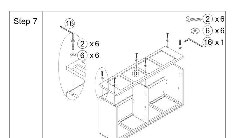
Attach bottom board (D) to left side board (B), right side board (C) and middle clapboard (H) with long bolt (②) and washer (⑥).
