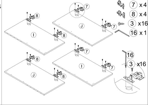
Install the big bend hydraulic door hinge( $\bigcirc$ ) on one of left side door (J) and right side door(I).Install middle bend hydraulic door hinge( $\bigcirc$ 8) on one of left side door (J) and right side door(I).
