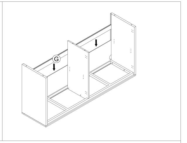
Insert slot (G) to left side board(B) and right side board (C).
