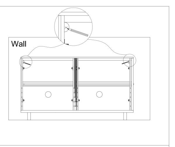
Place the sideboard against the wall. Mark the positions for the expansion plug on the wall.
