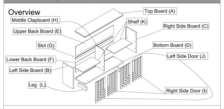
This <u>sideboard</u> has multiple parts and may require up to <u>45</u> minutes to assemble. To give you an overview of the <u>sideboard</u> parts, the above picture is to help you put the various parts into perspective. Please read through the instructions below to familiarise yourself with the parts and steps before assembly.
