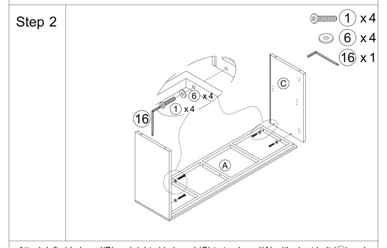
Attach left side board(B) and right side board (C) to top board(A) with short bolt (1) and washer(6).
