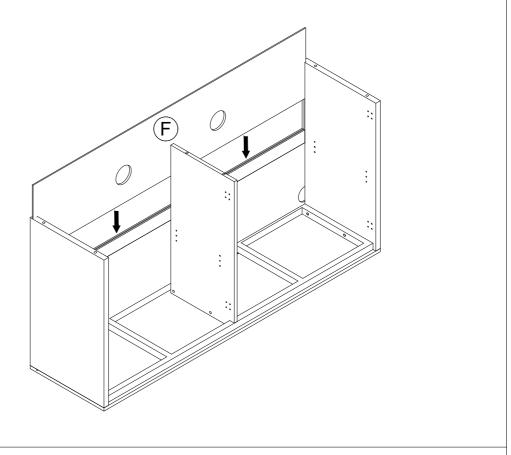
Insert lower back board (F) to left side board(B) and right side board (C).
