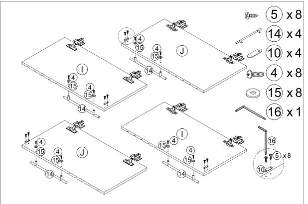
Attach handle (1) to left side door (J) and right side door (I) with screw (4) and washer (15). Attach magnetic door catch metal sheet (10) to left side door (J) and right side door (I) with screw (5).
