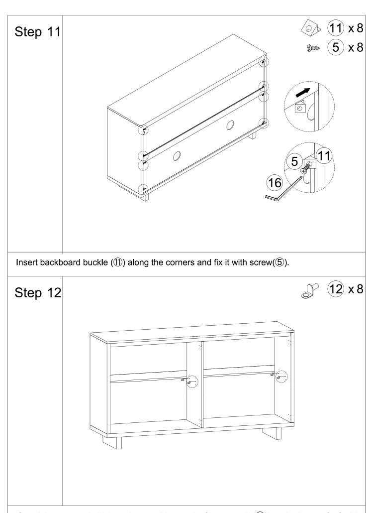
Stand the mounted sideboard up, and insert shelf support  $pin(\mathfrak{D})$  into the holes of left side board(B), right side board (C) and middle clapboard(H).
