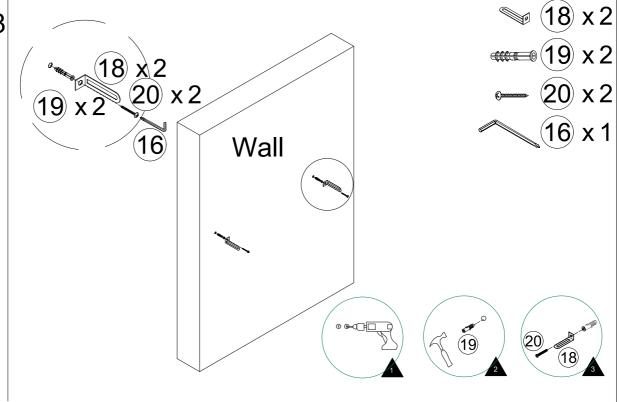
Drill holes on the wall in marking position, insert expansion plug((9)) into the holes, align with the expansion plug((9)),install the short side of Anti-Tip wall bracket((18)) with long screw((20)).
