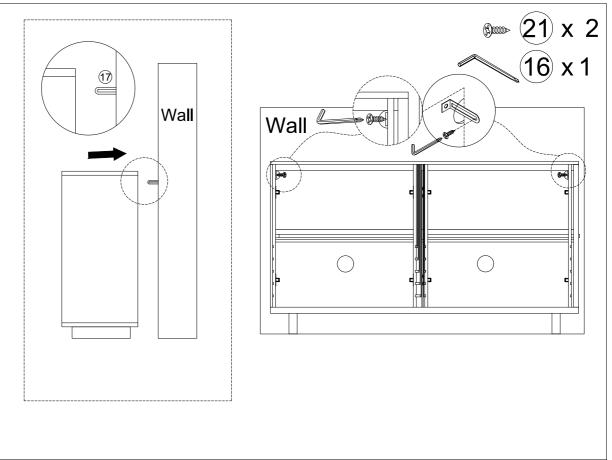
Attach the long side of Anti-Tip wall bracket(1) to left side board (B) and right side board (C) with short screw(2).
