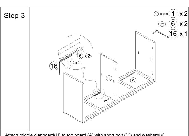
Attach middle clapboard(H) to top board (A) with short bolt (1) and washer(6).
