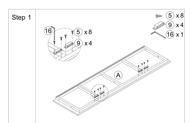
Attach magnetic door catch(9) to top board (A) with screw (5).
