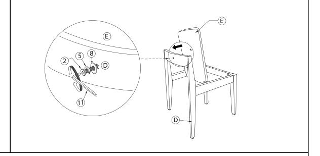
Install the Cushion Back (E) into Chair Back (D) using JCBC Screw (M6\*30) ②,Spring Washer (M6)⑤ and Flat Washer (M6\*13) ⑧ with Allen Key (M4) ① as pictured above.
