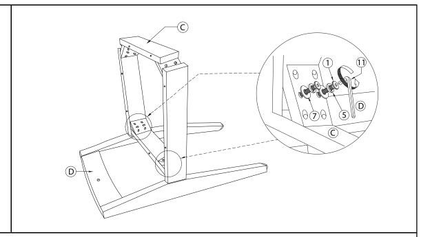
Place the Chair back (D) on a clean, non marring surface. Install the Box Seat (C) into the Chair back (D) using JCBC Screw (M6\*90mm) ①, Spring Washer (M6) ⑤, Flat Washer (M6) ⑦, with Allen Key (M4) ① as pictured above.
