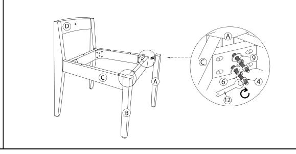
Install both Right Front Legs (A) and Left Front Leg (B) consecutively on both sides into the Box Seat (C) using Hex Nut (M6) 4, Spring Washer (M8) 6, Flat Washer (M8) 9 with Y Spanner M5(13) 12 as pictured above.
