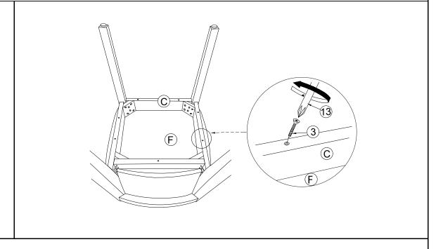
Place the assembled chair downside as shown. Install the Cushion Seat (F) onto the Box Seat (C) using CSK Screw (M4\*32) (3) with Screwdriver (13) as pictured above.
