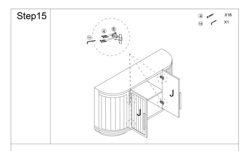
Attach hydraulic door hinge (6) of middle door(J) to left middle clapboard (F), right middle clapboard (G) with screw(4).
