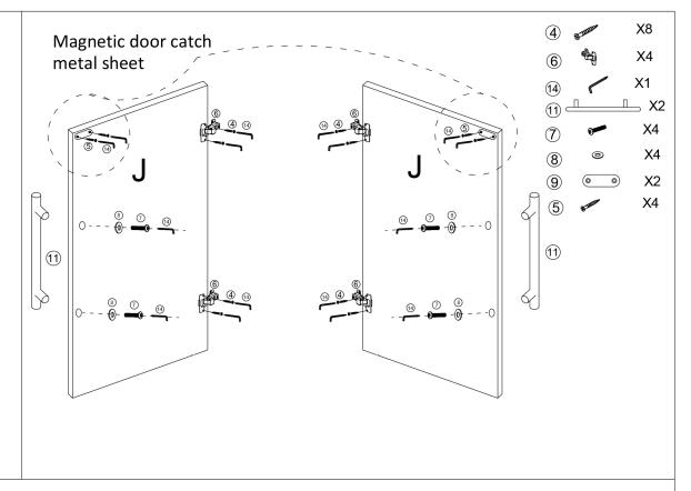
Attach hydraulic door hinge(6) to middle door(J) with screw(4). Attach handle(1) to middle door(J) with screw (7) and washer (8). Attach magnetic door catch metal sheet(9) to middle door(J) with screw(5).
