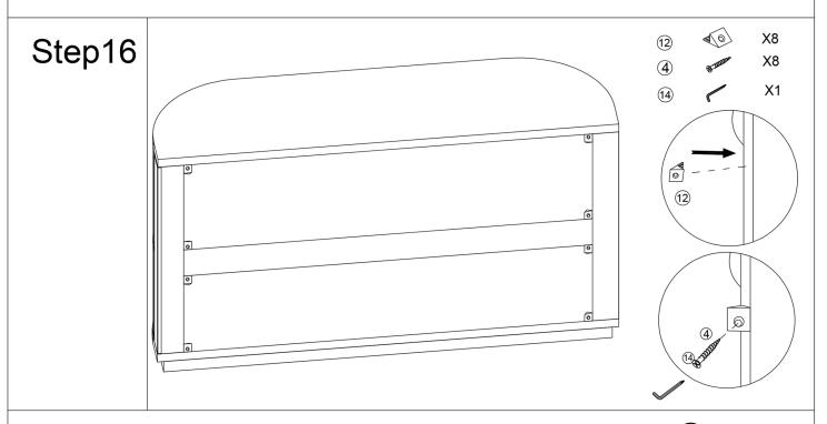
Insert backboard buckle ( $\mathfrak{D}$ ) along the corners and fix it with screw( $\mathfrak{A}$ ).
