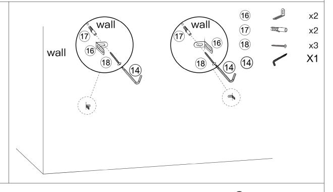
Drill holes on the wall in marking position, insert expansion plug(17) into the holes, align with the expansion plug(17), install the short side of Anti-Tip wall bracket(16) with long screw(18).
