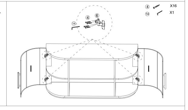
Attach hydraulic door hinge ( $\bigcirc$ ) of side door (I) to left side column(K), right side column(L) with screw( $\bigcirc$ ).
