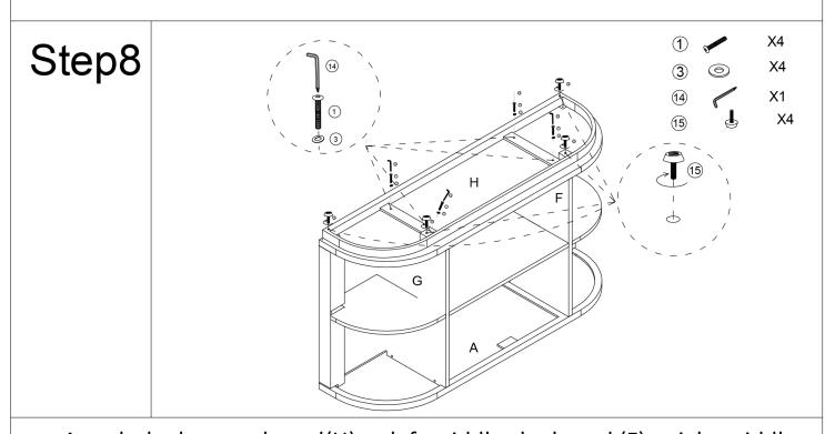
Attach the bottom board(H) to left middle clapboard (F). right middle clapboard (G) with bolt ( $\bigcirc$ 1) and washer( $\bigcirc$ 3). Screw adjustable leveling glide ( $\bigcirc$ 5) to bottom board (H).
