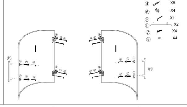
Attach hydraulic door hinge(6) to side door(I) with screw (4). Attach handle(1) to side door(I) with screw (7) and washer (8).
