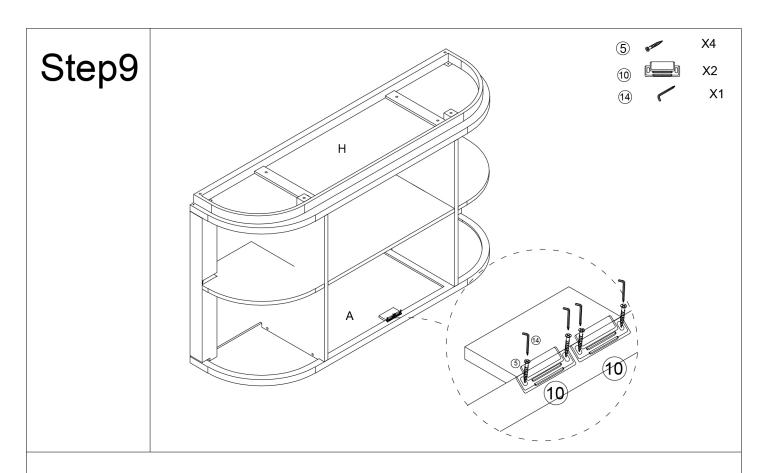
Attach magnetic door catch(10) to top board(A) with screw (5).
