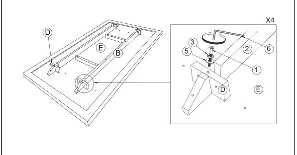
Insert U-Shaped Block (D) on the Table Rail (B) and install it using JCBC Screw (M6\*60) 1, Spring Washer (M6) 3, Flat Washer (M6\*13) 5 with Allen Key (M4x95) 6.
