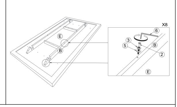
Place Table Rail (B) by following hole markings on the Table Top (E) and install it using JCBC Screw (M6\*45)②, Spring Washer (M6)③, Flat Washer (M6\*13)⑤ with Allen Key (M4x95)⑥.
