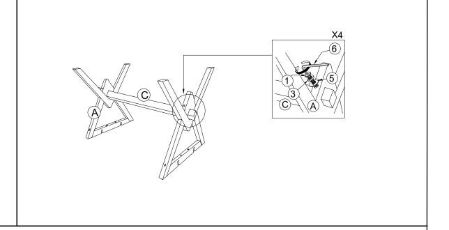
Install the Table Center Rail (C) into both Table Leg Frame (A) using JCBC Screw (M6\*60) ①, Spring Washer (M6) ③, Flat Washer (M6\*13) ⑤ with Allen Key (M4\*95) ⑥ as pictured above.
