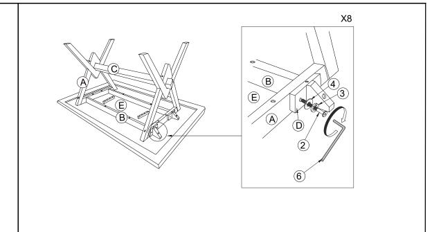
Install the U-Shaped Block (D) on the Table Leg (A) using JCBC Screw (M6\*45)  $\bigcirc$ , Spring Washer (M6)  $\bigcirc$ , Flat Washer (M6)  $\bigcirc$  with Allen Key (M4\*95)  $\bigcirc$ 6 as pictured above.
