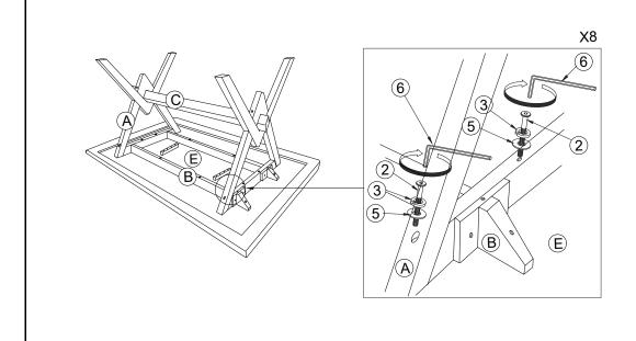
Install both Table Leg (A) into Table Top (E) using JCBC Screw (M6\*45) (2), Spring Washer (M6) (3), Flat Washer (M6\*13) (5) with Allen Key (M4\*95) (6) as pictured above.
