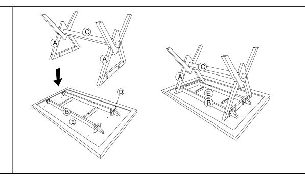
Place the assembled Table Leg (A) and Table Center Rail (C) onto the Table Top (E) by following the hole marking as pictured above.
