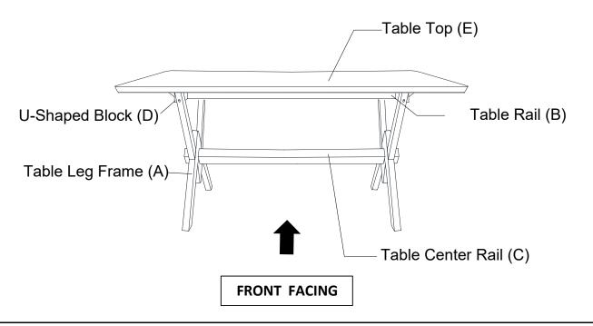
This Table has multiple parts and may require up to some 30 minutes to assemble. To give you an overview of the table parts, the above picture is to help you put the various parts into perspective. Please read through the instructions below to familiarise yourself with the parts and steps before assembly.
