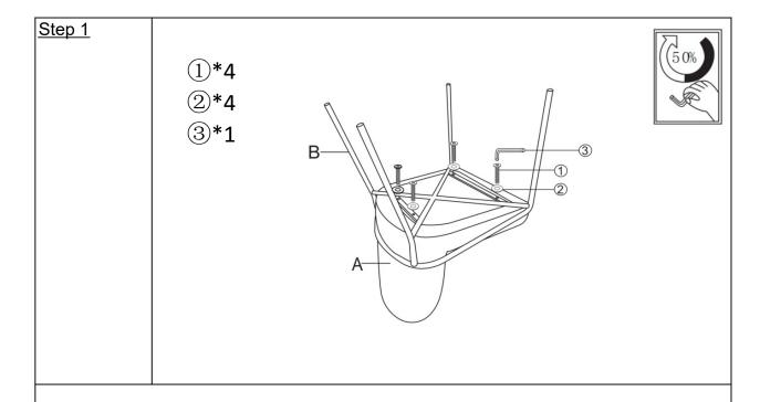
Attach the Frame (B) to Seat (A) using the Bolt  $(\mathfrak{D})$  and Washer  $(\mathfrak{D})$  with Allen Wrench  $(\mathfrak{D})$  as shown above.
