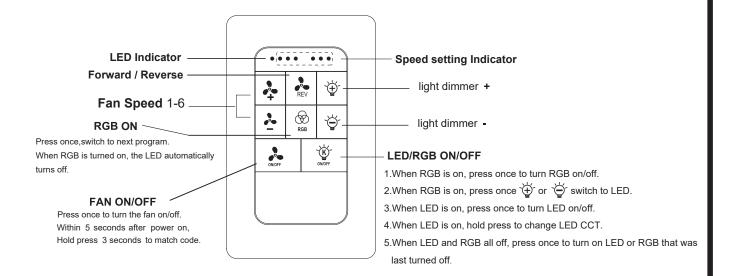
Within 5 seconds after power on, hold press + 3 seconds to clear code.
