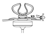
Remove 3 screws from the light kit, and then connect 2 sets of connectors.
