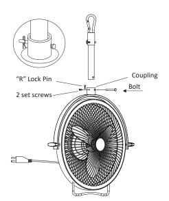
Insert the downrod into the coupling.
