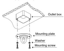
Secure mounting plate to outlet box by tightening 2 mounting screws & 2 washers.
