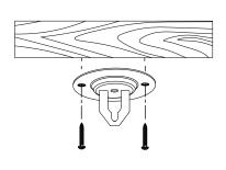
Secure mounting plate to wood ceiling by tightening 2 self tapping screws.
