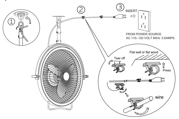
Feed the motor wire through inside the carabiner, hang the fan into mounting plate.
