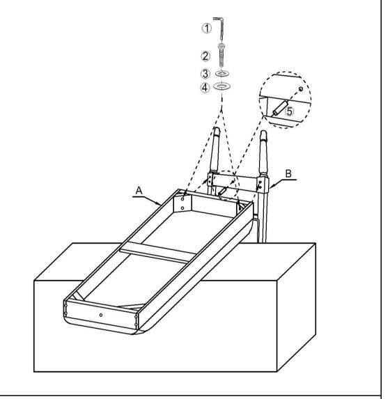
You will now have the Bench(A) bottom and the Legs(B) facing upwards. Insert the Legs(B) completely vertical into the seat frame corner then attach them using Bolts (②)+ Spring Washers(③)+Flat Washers(④)and the Allen Wrench(①) and Wood tenon(⑤).
