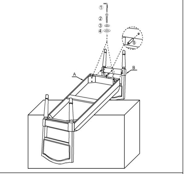
You will now have the Bench(A) bottom and the Legs(B) facing upwards. Insert the Legs(B) completely vertical into the seat frame corner then attach them using Bolts (2)+ Spring Washers(3)+Flat Washers(4)and the Allen Wrench(1) and Wood tenon(5).
