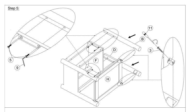
5.Attach the assembly just completed in step 4 to the Cabinet vertical bars (B) and Cabinet vertical bars(D) using Bolt 5 and Allen wrench 9, and attach the Compartment frame (H) using Vis 3.5x15mm 3 and Screwdriver (11).
