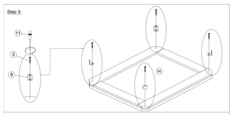
3.: Connect the Steel Bracks (8) to the Compartment frame(H) using Vis 3.5x15mm(3) and screwdriver (11).
