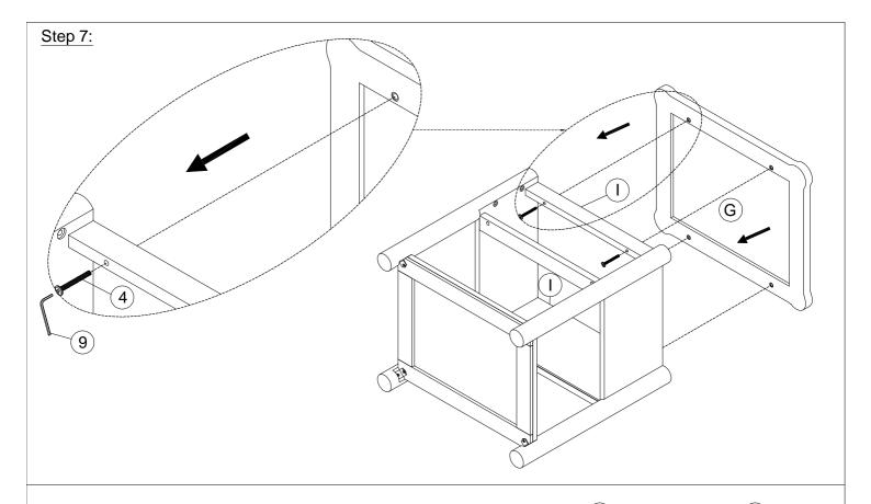
7:Attach the cabinet top (G) to the assembly completed in step 6 using Bolt 4 and Allen wrench 9 as shown in the image.
