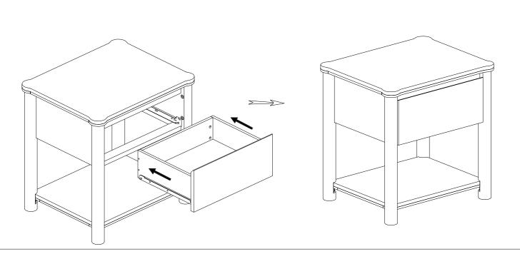
Inspect the Night stand an make sure all parts are adequately connected. Adjust the Levelers to desired height to avoid wobbles. Your Night stand is ready for use.
