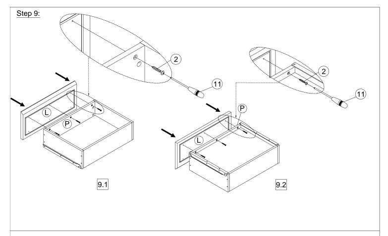
9:Assemble the main side of the drawer (L) to the assembly completed in step 8 using Vis  $\emptyset$ 4x20mm (2) and Screwdriver (11) as shown in the illustration.
