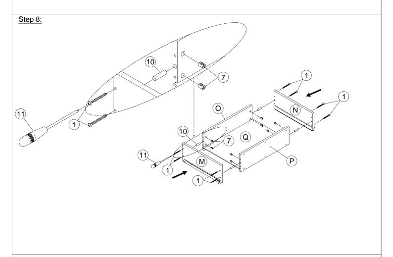
8:Assemble the drawer side (P), left side of the drawer (M), right side of the drawer (N),back of drawers (O), and drawer bottom board (Q) using Vis  $\emptyset$ 4x38mm 1, 7 and screwdriver 1 as shown in the diagram.
