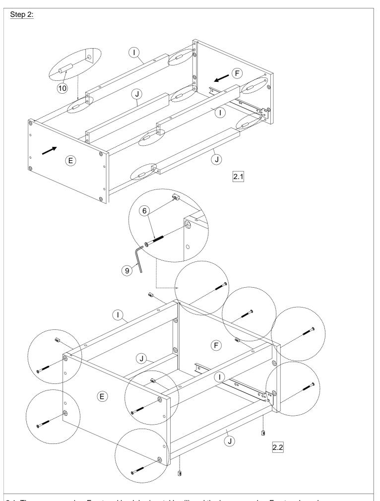
2.1: The upper crossbar Front and back horizontal bar(I) and the lower crossbar Front and rear lower crossbar(J) are attached to the Left hip plank (E), Right hip board (F) using Wooden dowel 10.
