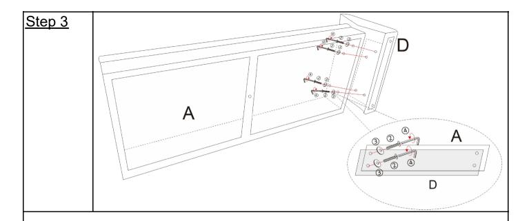
Align the hole on the right side of Seat Board(A) with Right Armrest (D), and use Allen Wrench (4) to tighten Gaskets(3) and Single Head Screw(2) in sequence. This step will tighten Single Head Screw(2).
