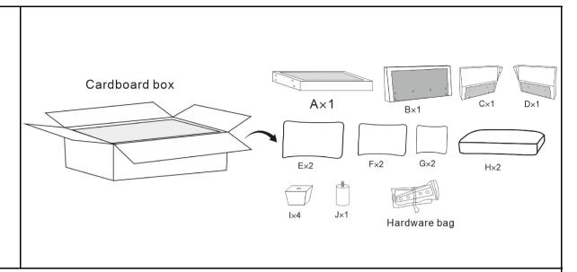
Remove Seat Board (A), Backrest (B), Left Armrest (C), Right Armrest (D), Headrest (E), Large Cushion (F), Small Cushion (G), Seat Cushion (H), Leg (I), Middle leg (J) and the corresponding hardware package from the carton and place them on a flat, clean surface without any dents.
