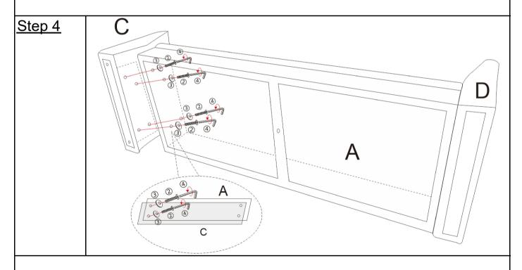
Align the hole on the Left side of Seat Board (A) with Left Armrest (C), and use Allen Wrench (4) to tighten Gaskets (3) and Single Head Screw (2) in sequence. This step will tighten Single Head Screw (2).
