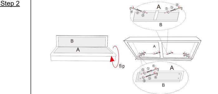
Align Seat Board (A) with Backrest (B) and flip it upside down. Align the holes at the bottom, and use Allen Wrench (4) to lock Gaskets (3) and Single Head Screw (1) together in sequence. Tighten Single Head Screw(1) in this step.
