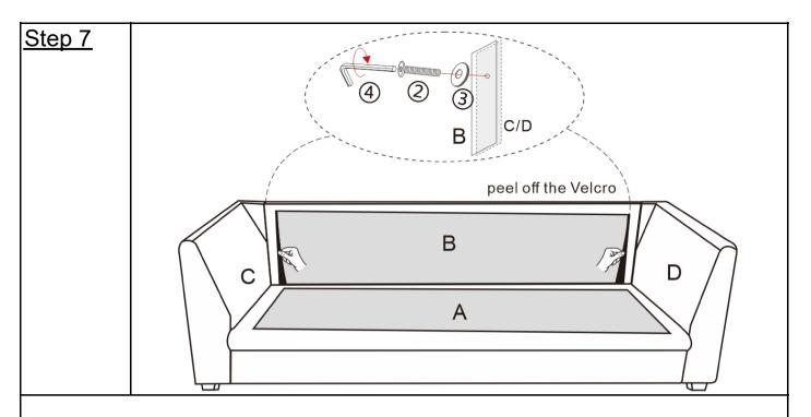
Unfasten the Velcro on both sides of Backrest (B), align the holes with Left Armrest (C), and use Allen Wrench (4) to tighten Gaskets (3) and Head Screw (2) in sequence.
