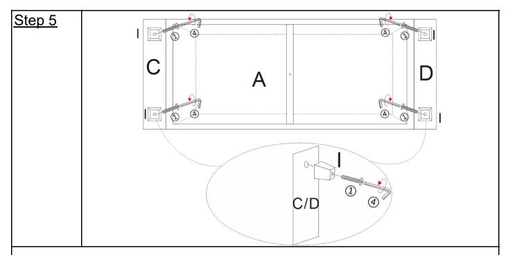
Lay the sofa flat, align Leg (I) with the holes at the top and bottom ends of Left Armrest (C) and Right Armrest (D), and use Allen Wrench (4) to tighten Single Head Screw (1). This step will tighten Single Head Screw (1).
