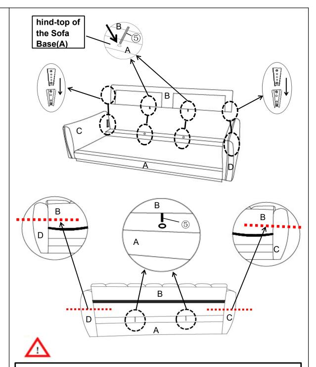
Especially Remind(very important!): When you push the Sofa Backrest (B) downwards and connect the both arms(C&D) and the mounting brackets of the Sofa Backrest (B), need to make sure the back side of Left Arm(C), Right Arm(D) and Sofa Backrest(B) on same plane;
