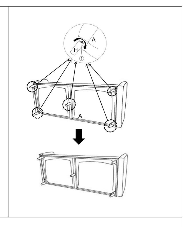
Install the Wood Legs(H) at the bottom of the Sofa by placing one Gasket(1) on the threaded stem.
