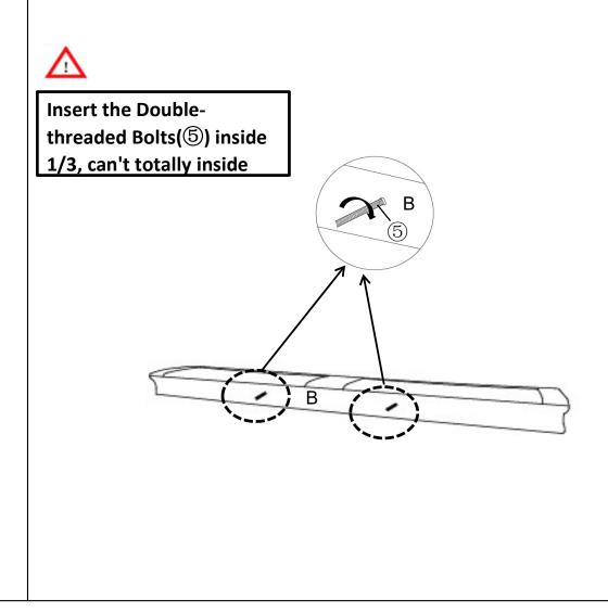
You will see two mounting positions on the bottom of Sofa Backrest(B), Insert the Double-threaded Bolts(⑤) into mounting positions and turn clockwise by hand until 1/3 inside (can't totally inside).
