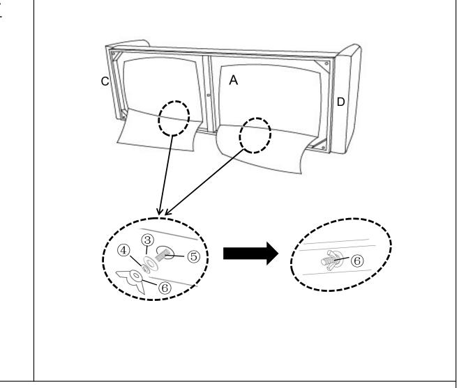
Position the rear side of the whole sofa on a clean, non-marring surface, place Washers( $\mathfrak{J}$ ) and Spring Washers( $\mathfrak{J}$ ) onto the Double-threaded Bolts( $\mathfrak{J}$ ), and secure using Wing Nuts( $\mathfrak{S}$ ).
