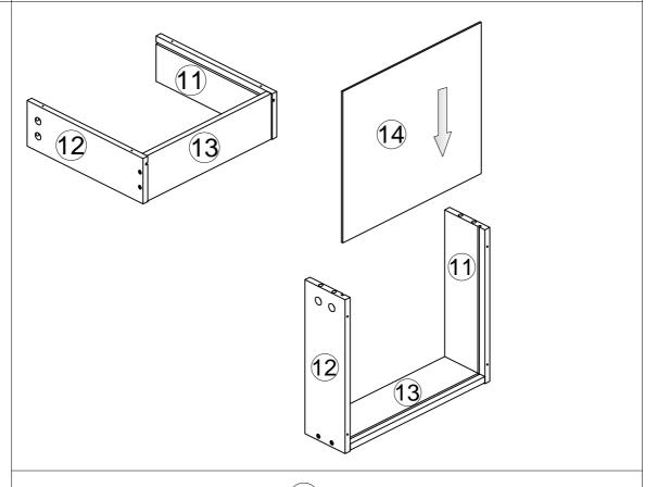
Attach Drawer Bottom Plate( 14) to the assembled unit from Step 15.
