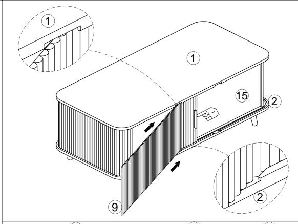
Push Door Panel (9) into the slot between Panel (1) and Base Plate (2). Be sure to pull the front end of the Door Panel to enter and support the other end with your hands. Pay attention to the direction of the door handle.
