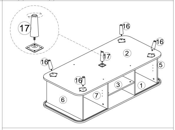
Fix Side foot(  $\widehat{16}$  )and Middle Foot(  $\widehat{17}$  )to the connecting iron plate.
