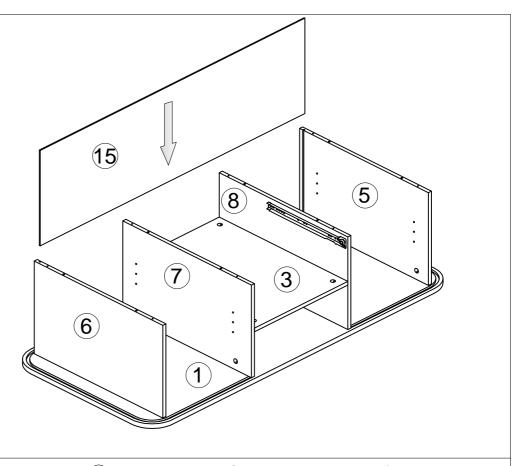
Attach Back Panel( 15) to the Panel ( 1), Left Side Panel( 5) and Right Side Panel( 6).
