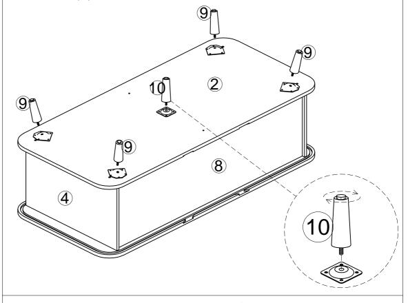
Connect Side foot(9) and Middle Foot(10) to the connectingiron plate.
