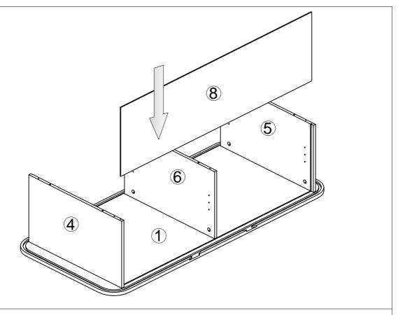
Attach Back Panel( 8 ) to the grooves of Panel( 1 ), Left Side Panel( 4 )and Right Side Panel( 5 )
