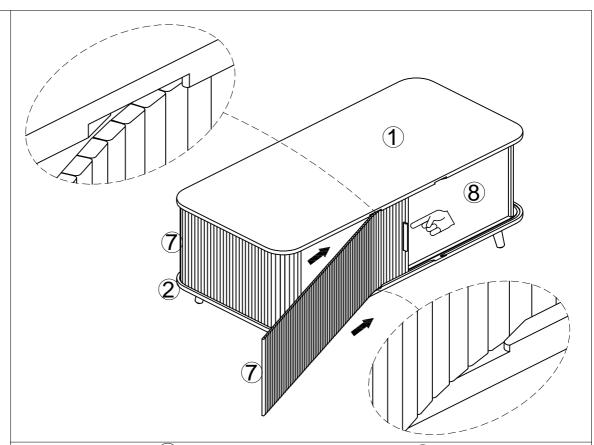
Push Door Panel (7) into the slot between Panel (1) and Base Plate (2). Be sure to pull the front end of the Door Panel to enter and support the other end with your hands. Pay attention to the direction of the door handle.
