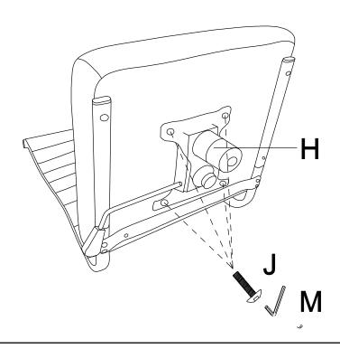
Assemble armrests Gx2 with the seat and back via Screws L. Turn the screws and finish with Allen Wrench M. Notice: Tighten all the screws completely.
