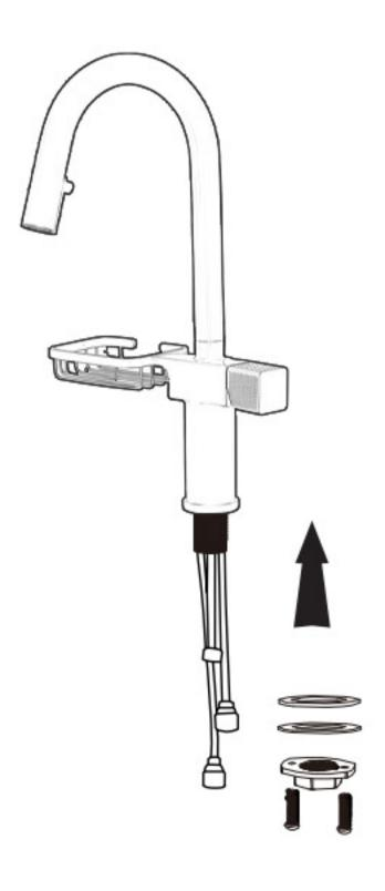
3. Insert the faucet into its mounting hole. From beneath the sink, slide the brass spacer back onto the faucet body. Thread the locknut back onto the threaded shank until hand-tight to secure. Finish tightening using an adjustable wrench.
