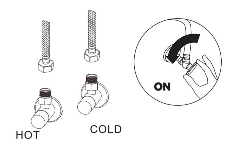
8. Turn the faucet on and ensure that there are no leaks. Check to ensure that both hot and cold water are running properly. Turn on the hand sprayer function and allow the sprayer to run for another 60 seconds, and check for any leaks.
