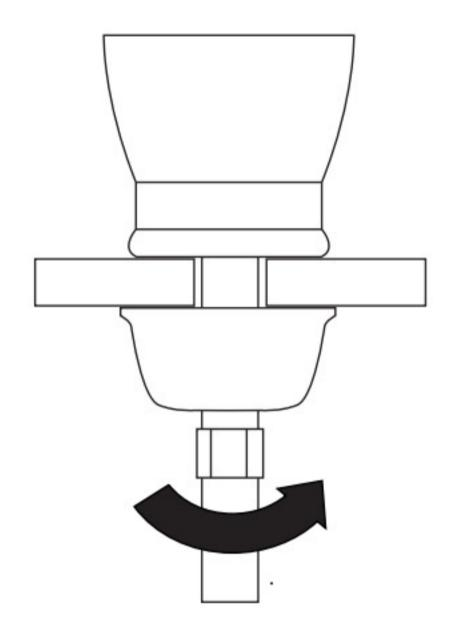
4. Attach the sprayer hose to its copper mounting post as shown. Insert the provided rubber O-ring into the lock nut before securing. Apply a bit of thread sealant or plumber's tape to the threads before tightening.
