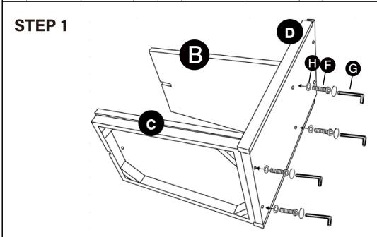
Place the back panel D on its side(long edge down) on a stable surface. Attach middle shelf B and bottom shelf C to the back panel with screws and flat washers as shown.
