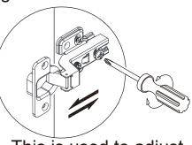
This is used to adjust front and rear.
