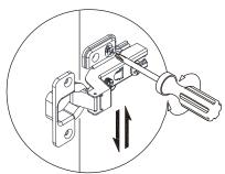
This is used to adjust and down direction.
