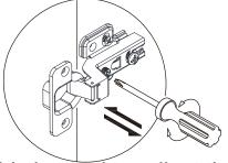
This is used to adjust the the door panel in the up door panel in the left and the door panel in the right direction.
