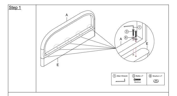
Fix the Head board A to the Base board E with Bolts ③ and Washer ⑥ by using Allen Wrench ①.
