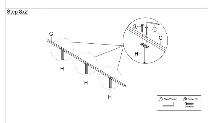
Fix the Middle support leg H to the Center support bar G with Bolts ③ by using Allen Wrench ①.
