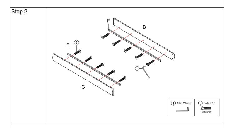
Fix the Side rails support bar F to the Side rail B and Side rail C with Bolts ③ by using Allen Wrench ①.
