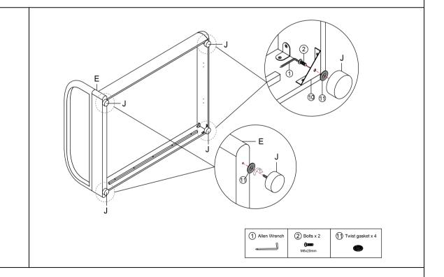
Fix the leg J to the Base board E and Metal Corner (10) with Bolts (2) and Twist gasket (11) by using Allen Wrench (1).
