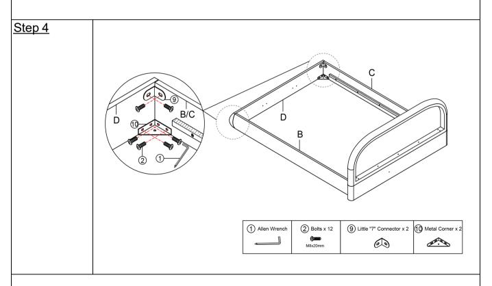
Fix the Foot board D to the Side rail B and Side rail C with Bolts ② ,Little "7" Connector ⑨ and Metal Corner ⑩ by using Allen Wrench ①.
