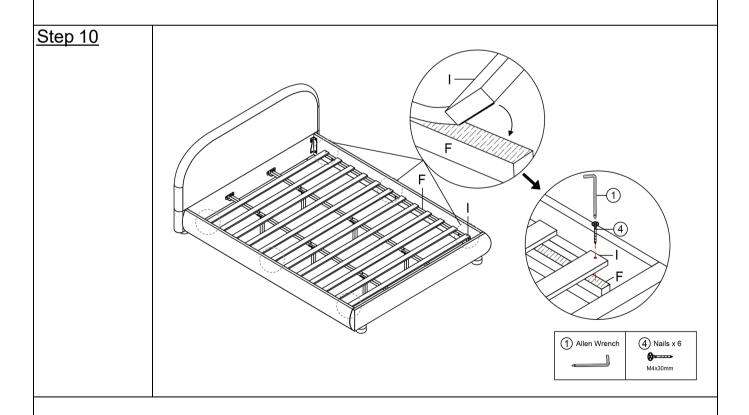
Fix the Slats I to the Side rails support bar F with Nails ④ by using Allen Wrench ①.
