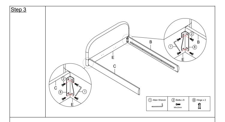
Fix the Side rail B and Side rail C to the Base board E with Bolts ② and Hinge ⑧ by using Allen Wrench ①.
