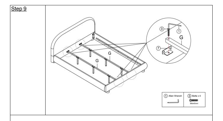
Fix the Center support bar G to the Center support bar fittings ⑦ with Bolts ③ by using Allen Wrench ①.
