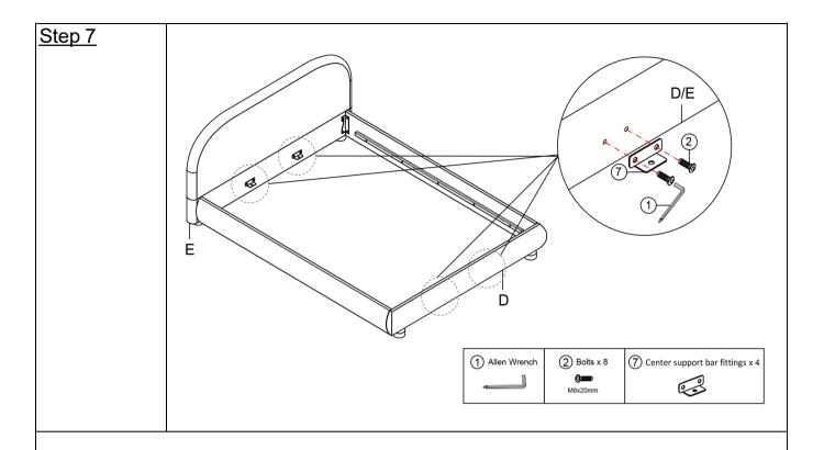
Fix the Center support bar fittings  $\bigcirc$  to the Foot board D and Base board E with Bolts  $\bigcirc$  by using Allen Wrench  $\bigcirc$ .
