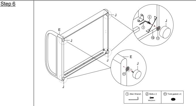
Fix the leg J to the Base board E and Metal Corner ⑩ with Bolts ② and Twist gasket ⑪ by using Allen Wrench ①.
