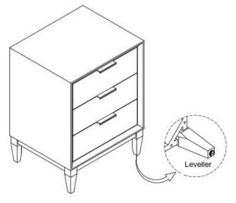
A Leveler is provided at the bottom of the leg to balance on uneven surface
