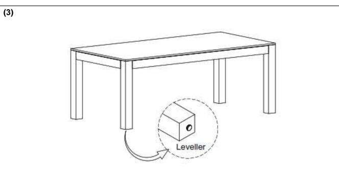
A Leveler is provided at the bottom of the leg to balance on uneven surface
