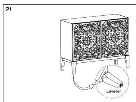
A Leveler is provided at the bottom of the leg to balance on uneven surface
