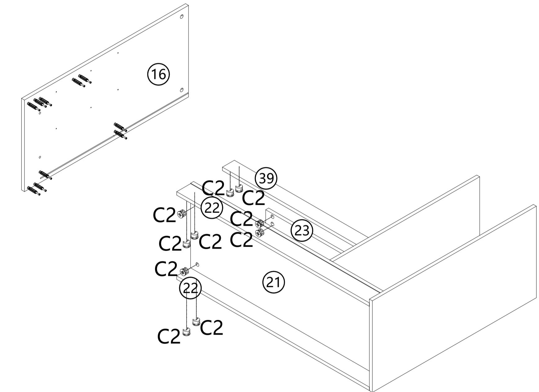
Make sure the arrow on the screw align to the hole on the side.
