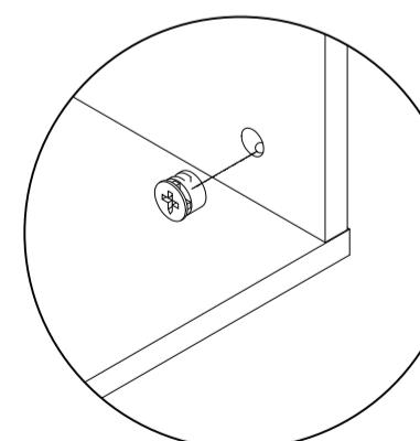
Make sure the arrow on the screw align to the hole on the side.
