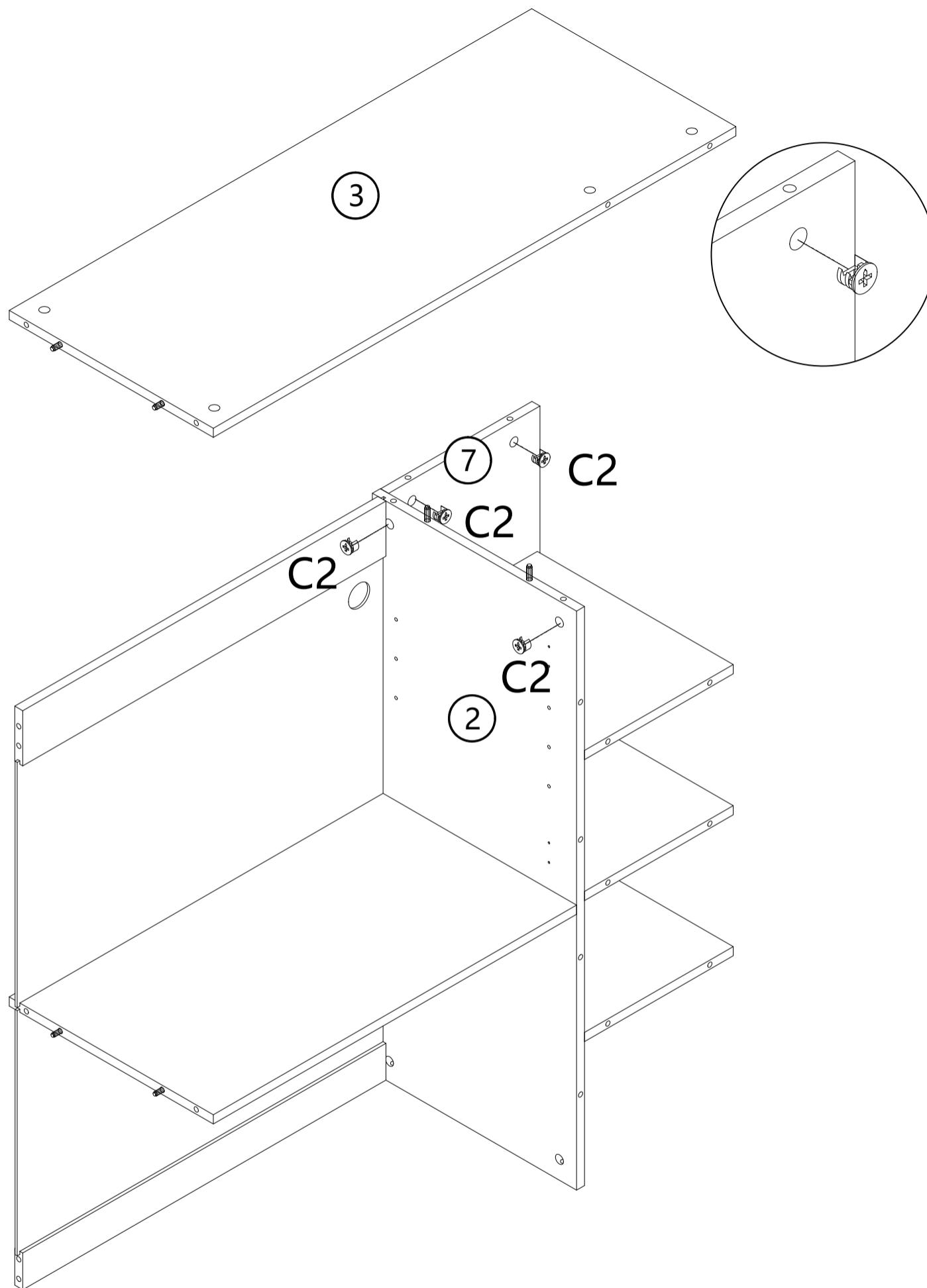
Make sure the arrow on the screw align to the hole on the side.
