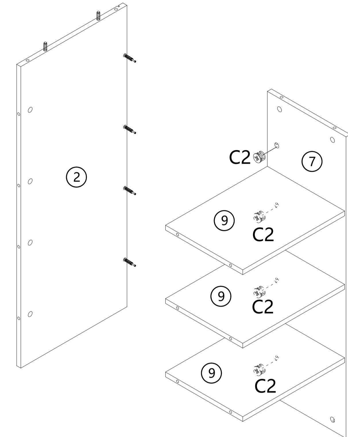
Make sure the arrow on the screw align to the hole on the side.
