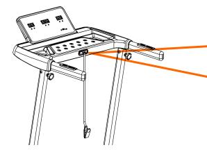
The color of the safety lock is red. In the plastic bag with the instruction manual, there is a red device with red rope, which is the safety lock. Insert the safety lock terminal in the yellow part of the instrument!
