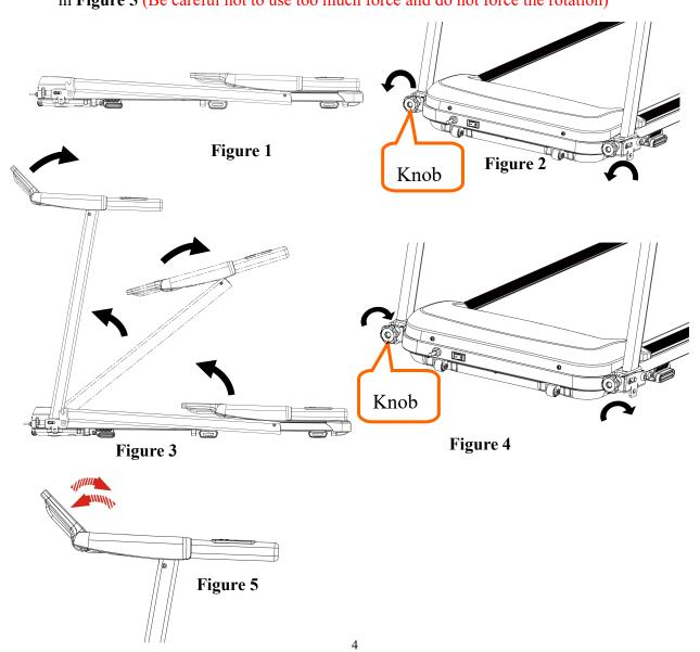
**Step 2.** Take out the plum knob and tighten it clockwise to lock the monitor on the column. Please note that you should gently hold the column tubes on both sides with your hands (when tightening the screws, be careful not to clamp the meter frame on the right column line). As shown in the following figure:
