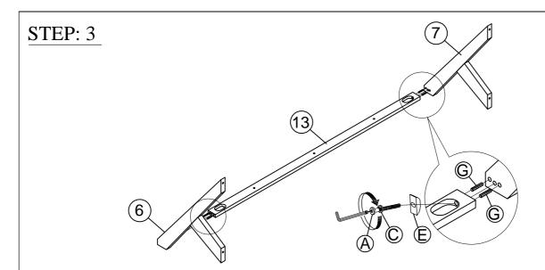
Assemble the support back headboard (13), into the left support headboard (6), the right support headboard (7) using the wooden dowel (G), bolt (A), Spring Washer (C), Washer (E), Allen key (I). Tighten all the bolts at this step.
