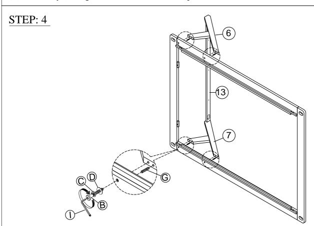
Assemble the part in step (3), into the part in step (2), using wooden dowel (G), bolt (B), Spring washer (C), flat washer (D), Allen key (I). Tighten all the bolts in this step.
