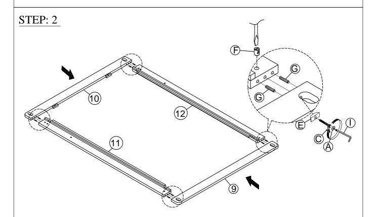
Assemble the left siderail (12), and the right siderail (11) to footboard rail (9), in step (1), and the headboard rail (10), using the wooden dowel (G), bolt (A), Spring Washer (C), curved washers (E), and horizontal-hole bolts (F). Tighten the bolts in this step.
