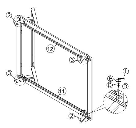
Assemble the Right legs (2), and the Left legs (3), into the Right siderail (11) and Left siderail (12), bolt (B), Spring washer (C), flat washer (D), Allen key (I). Tighten all the bolts in this step.
