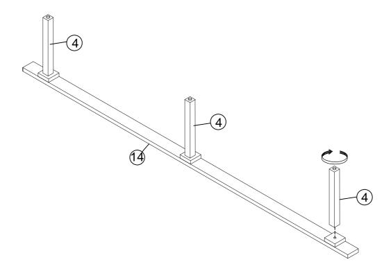
Assemble the support leg (4) into the Center support bar (14)
