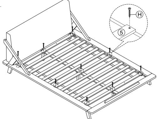
Assemble the slat (5) onto the Center support bar (14), Right siderail (11) and Left siderail (12), using Wood screws (H). Be careful not to tighten too much.
