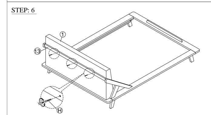
Assemble the headboard mattress (1), onto the support back headboard (13), and Wood screws (H). Be careful not to tighten too much.
