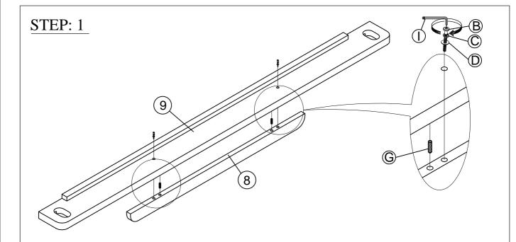
Assemble the support rail (8), to the footboard rail (9) using the wooden dowel (G), bolt (B), Spring Washer (C), flat washer (D), Allen key (I). Tighten all the bolts in this step.
