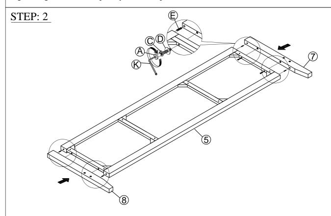
Attach the right footboard leg (7) and left footboard leg (8) to the frame headboard (5) using the bolts (A), spring washers (C), flat washers (D), and wooden dowels (E), Allen key (K) . Tightening the bolts completely at this step
