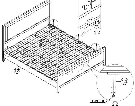
1.2 Assemble the slat (10) onto the siderails (12), using Wood screws (I). Be careful not to tighten too hard
