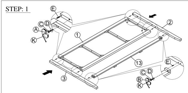
Attach the right headboard leg (3) and left headboard leg (2) to the frame headboard (1) using the bolts (A), spring washers (C), flat washers (D), and wooden dowels (E), Allen key (K).
