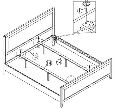
Assemble Center support bar (14) in step (6) to the support headboard (13) in step (1) and support footboard (9), in step (5), Wood screws (I). Be careful not to overtighten.
