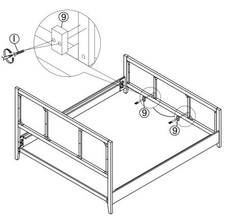
Assemble the support footboard (9) onto the inside of the footboard, using Wood screws (I). Be careful not to tighten too hard.
