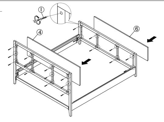
Assemble the headboard mattress (4) into the headboard step (1), assemble the footboard mattress (6), into the footboard step (2), Wood screws (I). Note: do not tighten too hard.
