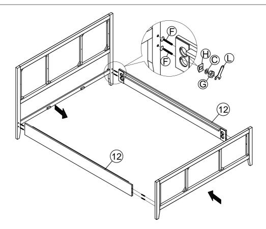
Assemble the siderails (12), to the headboard in step (1), and the footboard in step (2), using bolts (F), curved washers (H), Spring whasher (C), Hexagon nuts (G), and Wrench (L). Tighten all nuts in this step.
