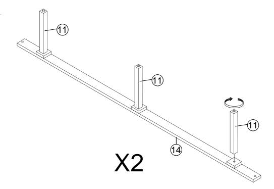
Assemble the support leg (11) into the Center support bar (14)
