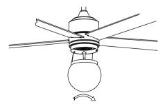
Slide the canopy up to ceiling and align the keyhole slots on the canopy with the 2 preassembled screws on the hanger bracket. Twist clockwise until it locks. Tighten two screws to fix the canopy securely.
