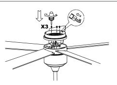
Remove 3 screws from motor.
