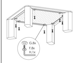
**Note:-**Bottom screws are to hold the marble top in position, do not over tight.
