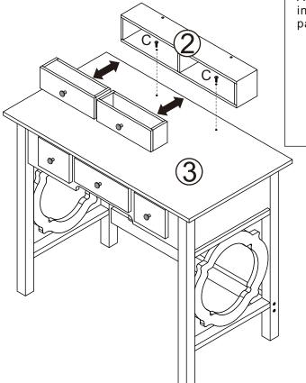
After all drawers are pulled out, install the handle on the drawer panel as shown in the picture below.
