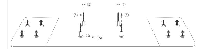
· Tighten the screws in order, place the washers, and then use a wrench to tighten the bottom small nut.
