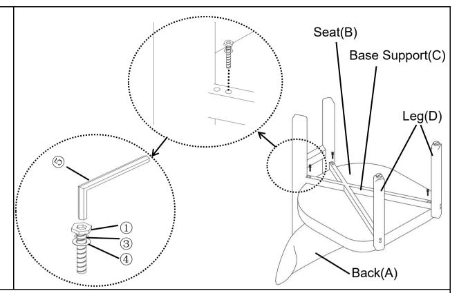
Attach the Seat(B) into the mounting positions of the Base Support(C) using Bolts(1), Spring Washers(3) and Washers(4) with the Allen Wrench(5). Do not fully tighten the Bolts.
