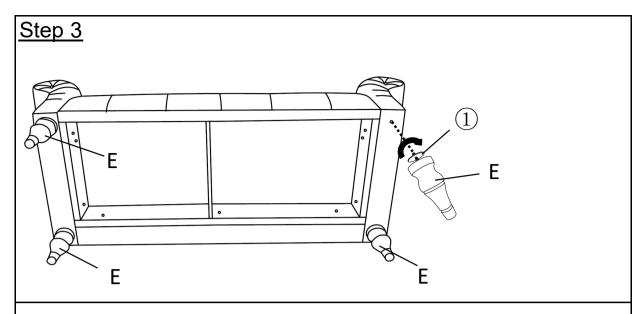
Assemble the Leg(E) to the Left Arm(C) and Right Arm(D)
