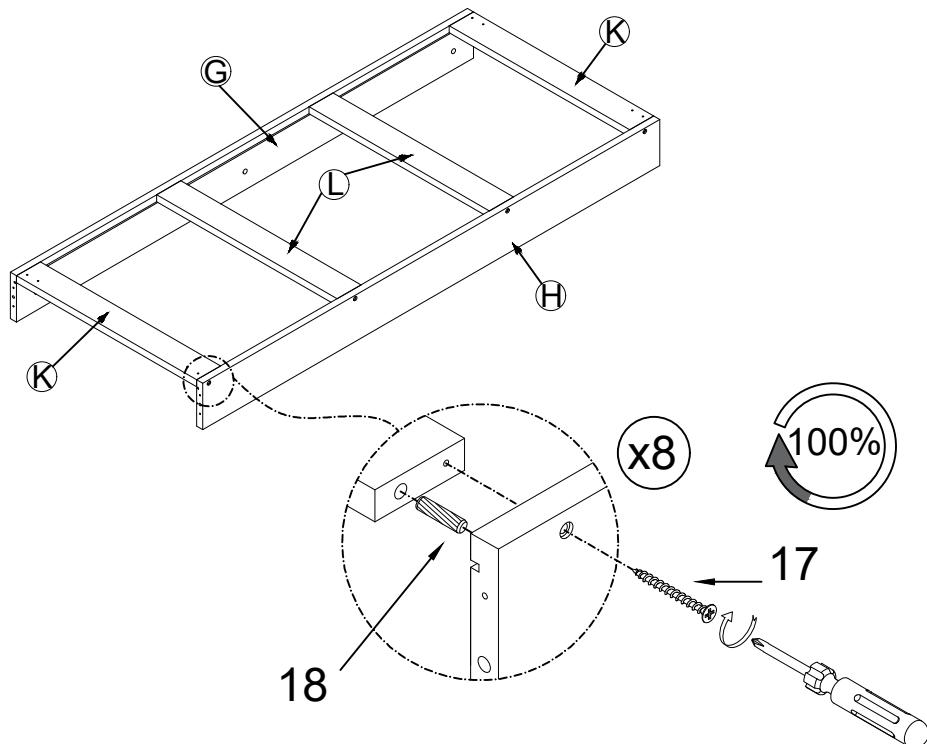
**Step 14:** Pass Drawer Bottom Panel (J) to in the Drawer Panel (H),(G) and Drawer Support Strip (K),(L).
