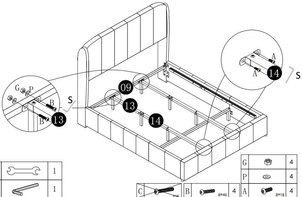
First, Find the tools Allen Wrench(S) and Spanner(Q) and use the Bolts(B) to assemble the Metal Brackets(J) into the Cross Slat With Mounting Position(⑨).Please repeat this step.
