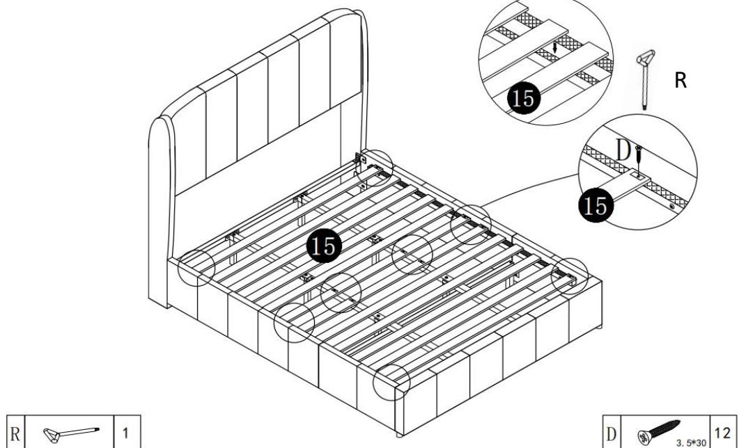
Assembly the Straight Slats(⑯),put the part on the frame,like above pic, and than use the Cross Wrench(R) to fix the Self-tapping screw(D) into the Side bars(Left ⑪&⑫ and right⑬&⑭) and Middle bar(⑯).
