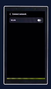
for wireless, turn WLAN toggle to On position, choose from WiFi network list, enter wireless network password
