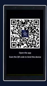
• once connected to Wireless Network, go into Starfish App, tap + in upper left corner, tap Scan, scan the QR code. Panel will bind to Starfish account. Once bound successfully, you can choose to upload all devices in all room, or devices from selected rooms.
