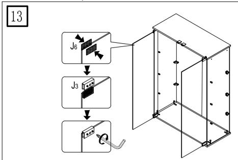
Use magnet [J3] and cushion [J6] to tighten screws to fix.
