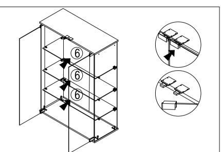
Put the glass shelf board into the main body while tilting it diagonally and place it on the dowel.
