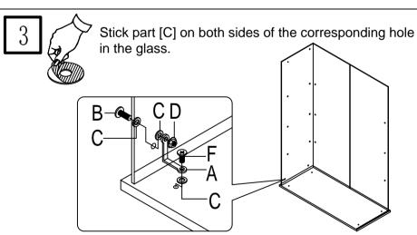
Align Fixing Parts [A] into the screw hole of the base plate[1], Temporarily tighten with screws [F]. Use screws [B],washers [C], nuts [D] in order in the hole (lead hole) on the glass (side), temporarily tighten fixing parts [A] and adjust the position. Finally, tighten all screws[B].
