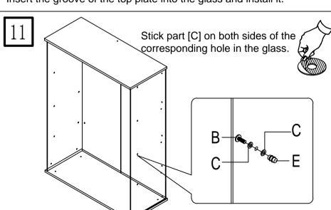
Use the washer [C] screws [B] to install the dowel [E] into the hole open on the side (lead hole).
