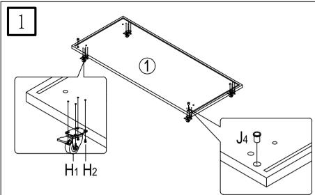
Attach the wheel parts [H] to [1] base plate. Attach the door holder [J4] to the [1] base plate.
