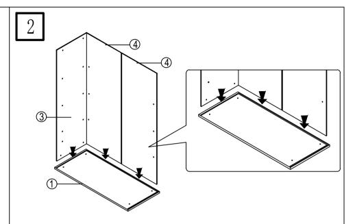
Insert the glass of  $[\mathfrak{A}]$  and  $[\mathfrak{A}]$  into the groove of  $[\mathfrak{A}]$  base plate.
