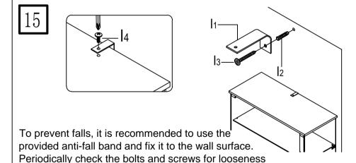
Mark 10mm below the height of the product, install the screw receiver [L2] on the wall, Secure the fall prevention band [L1] with screws [L3].
