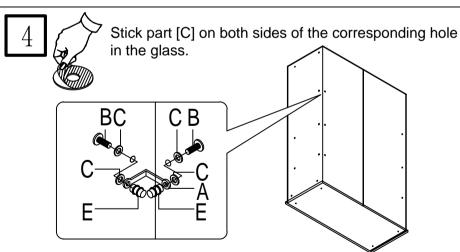
In the screw hole of the glass (side) Fixing parts [A], Temporarily tighten with dowels [E] .
