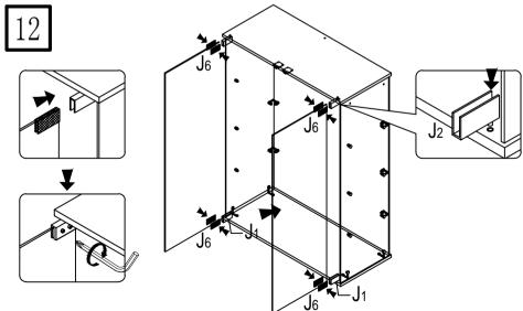
Door receiving metal fitting (lower part) [J1] cushion [J6] and Door receiving metal fitting (upper part) [J2] cushion [J6] Slide and insert, tighten screws to fix.
