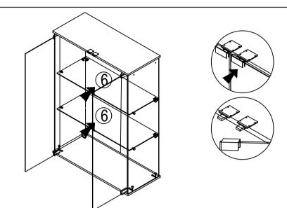
Put the glass shelf board into the main body while tilting it diagonally and place it on the dowel.
