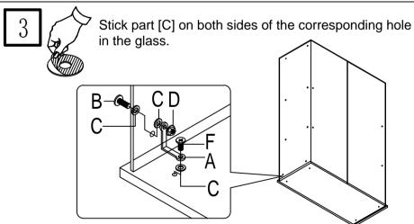
Align Fixing Parts [A] into the screw hole of the base plate [1], Temporarily tighten with screws [F]. Use screws [B], washers [C], nuts [D] in order in the hole (lead hole) on the glass (side), temporarily tighten fixing parts [A] and adjust the position. Finally, tighten all screws[B].
