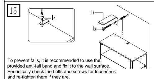
Place the product on the wall while pulling the attached anti-fall band
