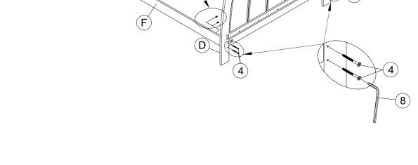
8.1:The assembly in step 7 connects to the assembly in step 5 using a wooden dowel 9 as shownin the image 8.2:After completing step 8.1, we connect the assembly using Bolt 4 and Allen wrench 8 as shown in the image.
