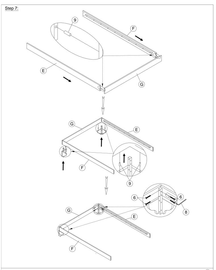
7.1:Attach the Left Side panel (E) and Right Side panel (F) to the Bed footboard (G) using Wooden dowel (9) as shown
