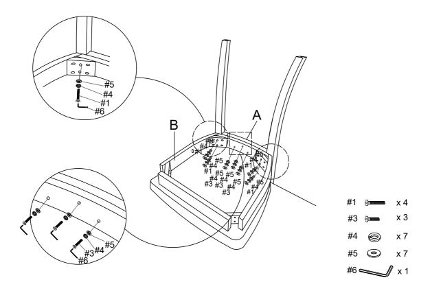
Step 2. Attach front legs (parts C) to seat frame (part B) using medium bolts (part #2), spring washers (part #4), flat washers (part #5) and allen wrench (part #6).
