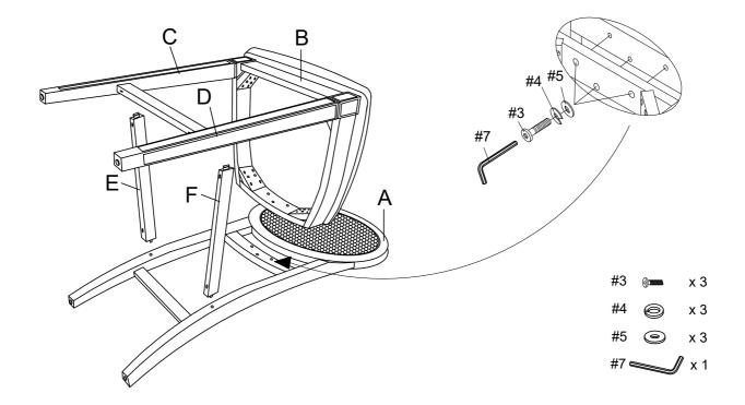
Step 3. Secure corners on seat frame (part B) to back frame (part A) using long bolts (part #1), spring washers (part #4), flat washers (part #5) and allen wrench (part #7).
